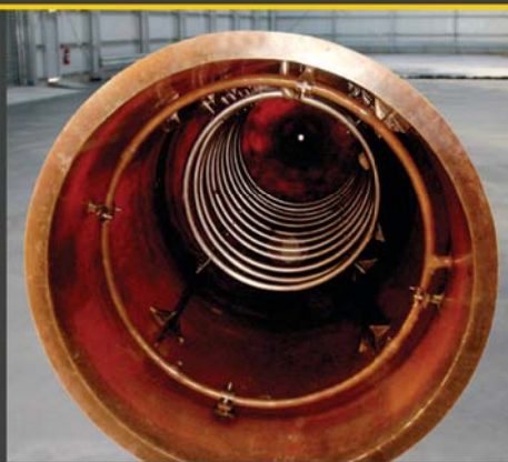
30 KL FRP Reaction vessel with coil and sparger
