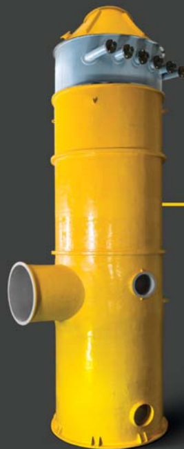
SO2 quench 2.9m diam x 13.8m height 2.3mm ECTFE + FRP
