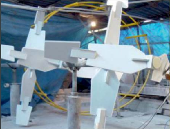
2.3mm MPTFE lining to MS agitator for 50 KL reaction vessel
