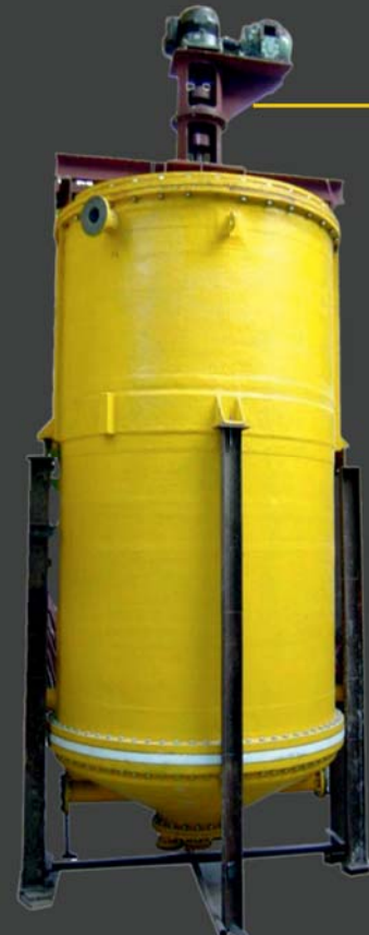
20 KL Reaction vessel
