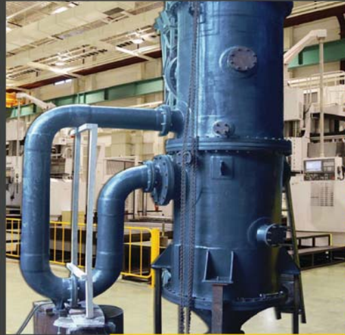
Spin Bath Solution Evaporator: \text{Na}_2\text{SO}_4 + \text{H}_2\text{SO}_4 + \text{ZnSO}_4 + \text{H}_2\text{O}
